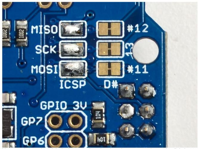
You can also cut the mini wire between the other three jumpers to 'release' the digital #11, 12 and 13 pins from being tied to the SPI pins. You can do this after you've gotten things working.
