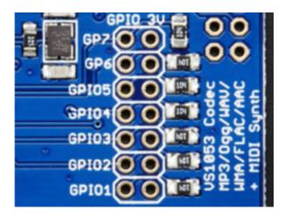
The VS1053 codec chip has 7 'General Purpose Input/Output' pins that you can use to detect button presses and/or light up a small LED. GPIO1 is also used to put it into MIDI mode. By default all these pins are pulled **low** to ground with 100K resistors. They are 3V logic level so if you want to attach a button, you can connect the two wires between the GPIO pin on the left and the 3V breakout on the right. If you don't want to use these pins just leave them be, they are not required for use!
