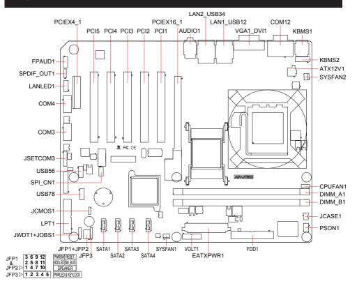
Figure 1: Board Layout - Jumper and Connector Locations
