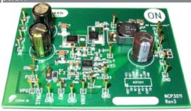
PowerGood pin to indicate that the system is in regulation. The dual function SYNC pin synchronizes the device to a higher frequency (Slave Mode) or outputs a 180° out-of-phase clock signal to drive another NCP3011 (Master Mode). Protection features include lossless current limit and short circuit protection, output overvoltage and undervoltage protection, and input undervoltage lockout.
