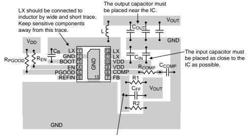
The voltage divider and compensation components must be connected as close to the IC as possible.
