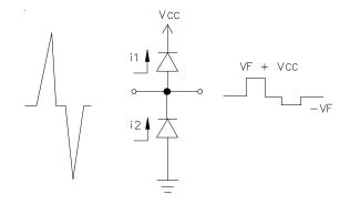
Figure 4 - "Rail-To-Rail" Protection Topology (First Approximation)
