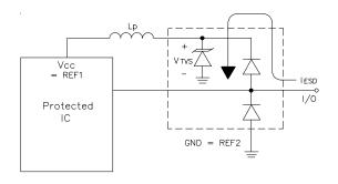
Figure 6 - Rail-To-Rail Protection Using RailClamp TVS Arrays
