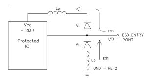
Figure 5 - The Effects of Parasitic Inductance
