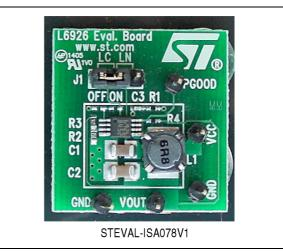
The low MOSFET R<sub>DS(on)</sub> ensures high efficiency at high output current.
