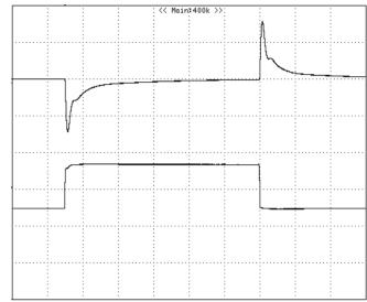
**Figure 8:** Output voltage response to step-change in load current (75%-50%-75% of lo, max; di/dt = 0.1A/ $\mu$ s). Load cap:  $10\mu$ F tantalum capacitor and  $1\mu$ F ceramic capacitor. Top Trace: Vout (50mV/div, 200 $\mu$ s/div), Bottom Trace: I out (5A/div). Scope measurement should be made using a BNC cable (length shorter than 20 inches). Position the load between 51 mm to 76 mm (2 inches to 3 inches) from the module
