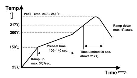
Note: The temperature refers to the pin of E48SR, measured on the pin +Vout joint.
