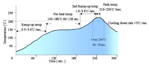
Note: The temperature refers to the pin of E48SR, measured on the pin +Vout joint.
