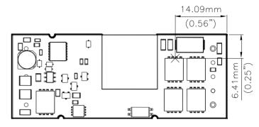
**Figure 21:** Hot spot temperature measured point The allowed maximum hot spot temperature is defined at 107  $^{\circ}$
