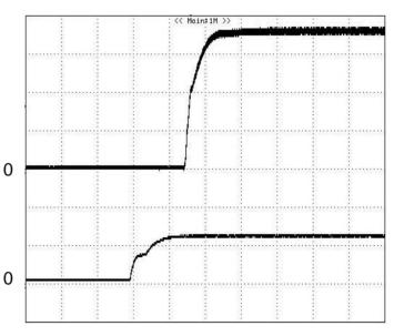
**Figure 7:** Turn-on transient at zero load current (2 ms/div). Vin=48V Top Trace: Vout, 0.5V/div; Bottom Trace: ON/OFF input, 5V/div
