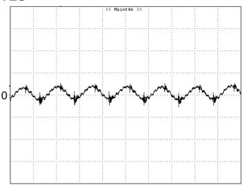
**Figure 11:** Input Terminal Ripple Current, i<sub>c</sub>, at full rated output current and nominal input voltage with 12μH source impedance and 33μF electrolytic capacitor (500 mA/div, 2us/div)
