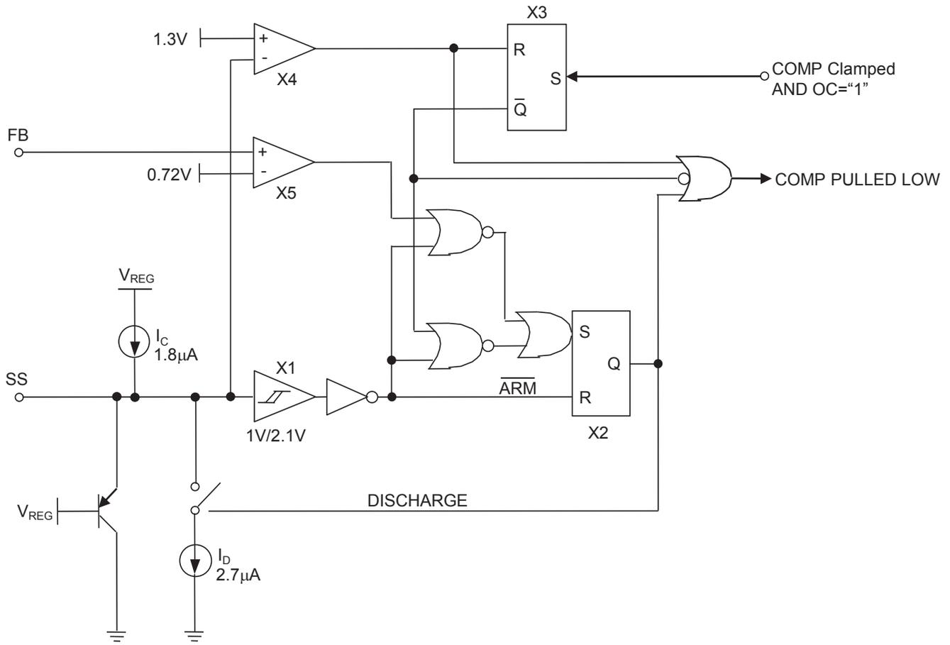
**Figure 3. Details of the Soft-start and Overload Hiccup Control Circuit**
