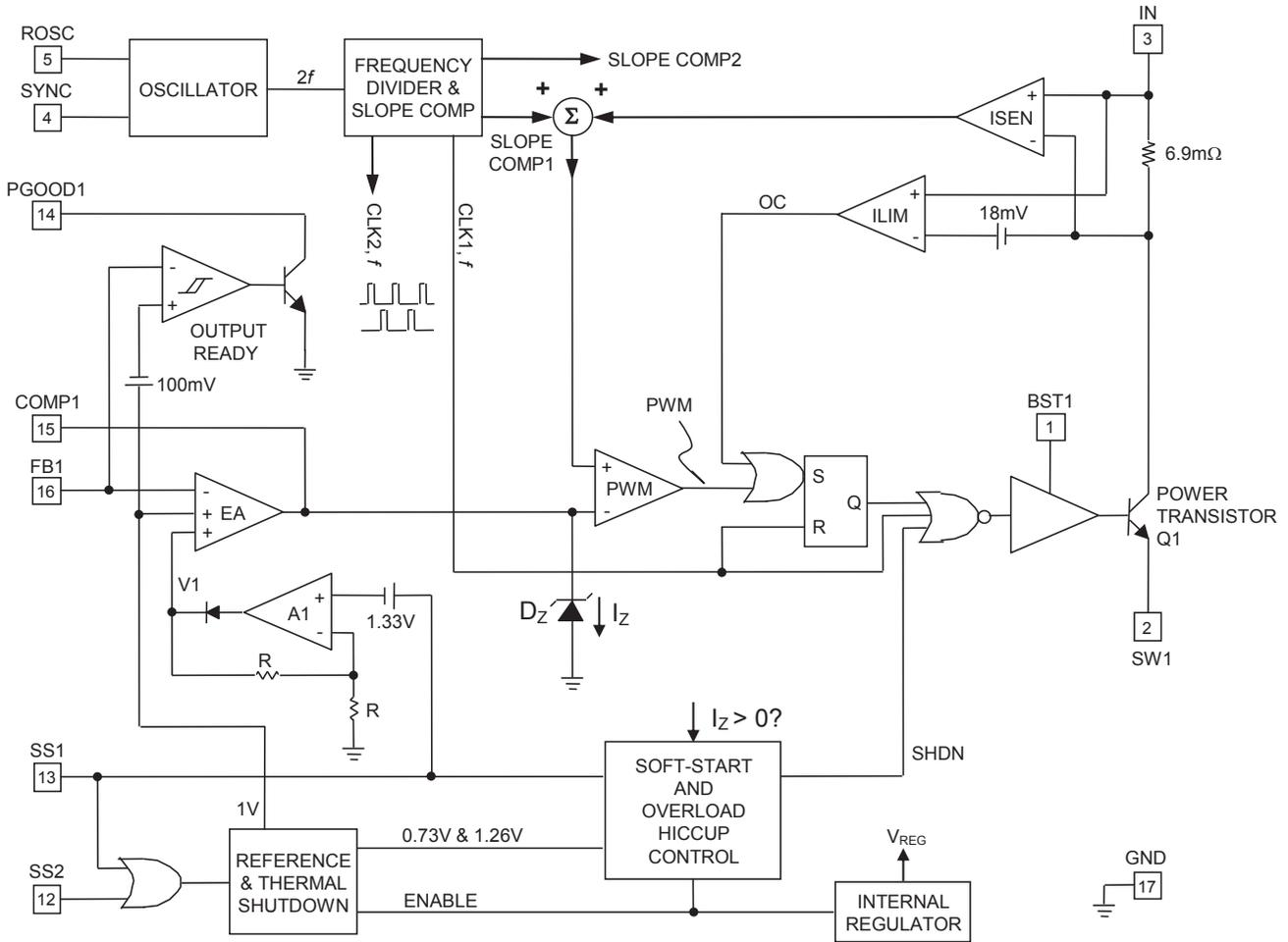
Figure 2. SC2440A Block Diagram (Channel 1 Shown)
