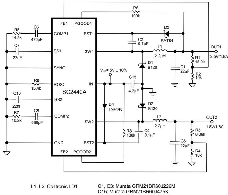
**Figure 17. 1.2MHz 5V to 2.5V and 1.8V Step-down Converter.**
