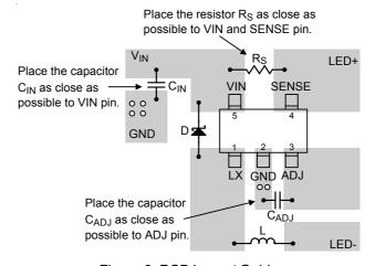
Figure 3. PCB Layout Guide
