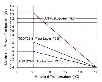
Figure 2. Derating Curve for Packages
