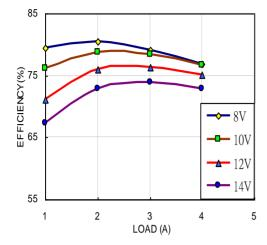
Figure 1: Converter efficiency vs. output current (0.90V output voltage)
