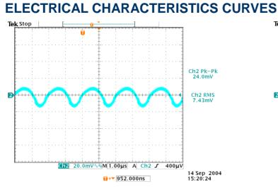
Figure 13: Output ripple & noise at 12 Vin, 3.3 V/4A out
