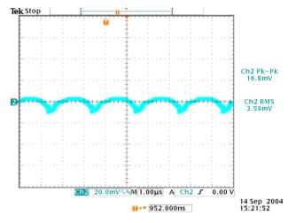
Figure 10: Output ripple & noise at 12 Vin, 1.5 V/4A out
