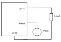
Figure 32: Circuit configuration for programming output voltage using external voltage source
