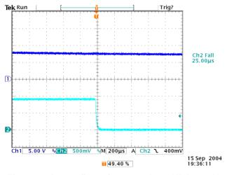
Figure 17: Power off waveform at 12vin, 0.9V/4A out with
