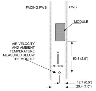
Figure 34: Wind tunnel test setup
