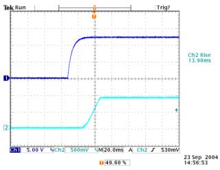
**Figure 15:** Power on waveform at 12vin, 0.9V/4A out with application of Vin
