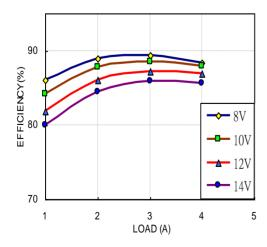
Figure 5: Converter efficiency vs. output current (2.5V 0utput voltage)
