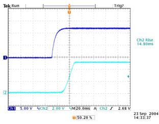
Figure 16: Power on waveform at 12vin, 5V/4A out with application of Vin
