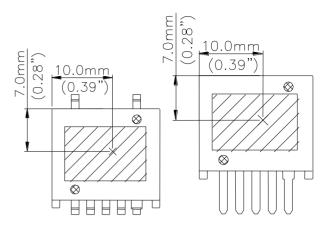
*Figure 35:* Temperature measurement location \* The allowed maximum hot spot temperature is defined at 113 C.
