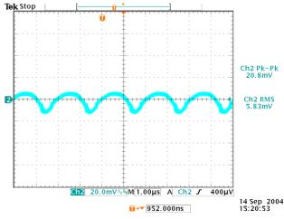
Figure 12: Output ripple & noise at 12 Vin, 2.5 V/4A out
