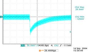
**Figure 24:** Typical transient response to step load change at 2.5A/µS from 50% to 100% of lo, max at 12Vin, 5.0V out (measurement with a 1uF ceramic and a 10µF tantalu)
