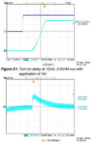
**Figure 23:** Typical transient response to step load change at 2.5A/µS from 100% to 50% of lo, max at 12Vin, 5.0V out (measurement with a 1uF ceramic and a 10µF tantalum)
