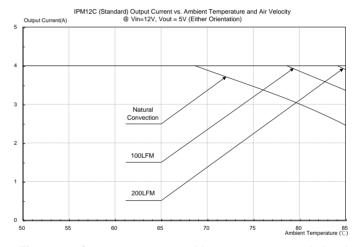
Figure 36: Output current vs. ambient temperature and air velocity @ Vin=12V, Vo=5V
