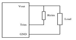
Figure 31: Trim down Circuit configuration for programming output voltage using an external resistor
