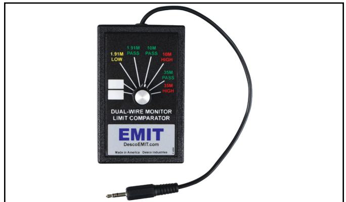
Figure 6. EMIT 50524 Limit Comparator for Dual-Wire Monitors
