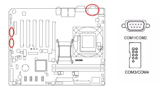
AIMB-767 supports four serial ports - three RS-232, and one RS-232/422/485 - COM3. The user can use JSETCOM3 to select RS-232/422/485 modes for COM3. These ports can connect to serial devices, such as a mouse or a printer, or to a communications network.
