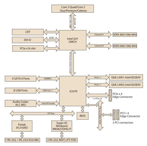
Figure 1.3 AIMB-767 Block Diagram
