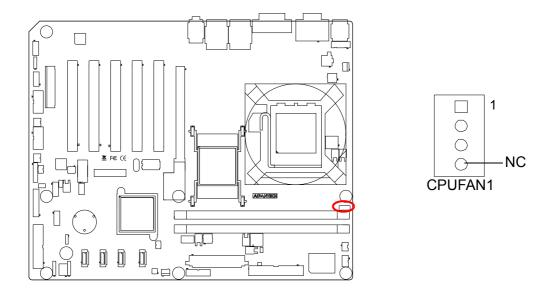
If a fan is used, this connector supports cooling fans of 500 mA (6 W) or less.
