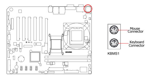
Two 6-pin Mini-Din connectors (KBMS1) on the motherboard provide connection to a PS/2 keyboard and a PS/2 mouse, respectively.
