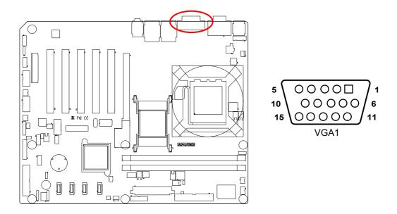
The AIMB-767 includes a VGA interface that can drive conventional CRT displays. VGA1 is a standard 15-pin D-SUB connector commonly used for VGA. Pin assignments for CRT connector VGA1 are detailed in Appendix B.
