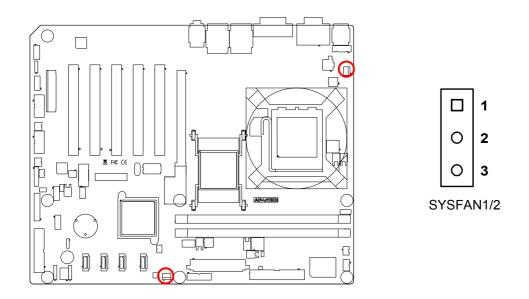
If a fan is used, this connector supports cooling fans of 500 mA (6 W) or less.
