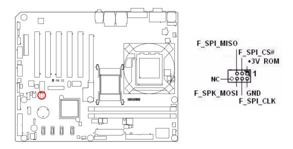
SPI flash card pin header can be used to flash the BIOS.
