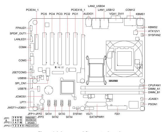
Figure 1.1 Jumper and Connector Location
