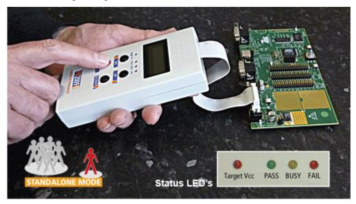
In 'Standalone Mode', the FS2009USB is controlled via the push buttons on the front panel of the programmer - no PC connection is required. The programmer LCD and the LED Status Indicators are used to display the current status of the programmer. It is possible to select from 1 of 64 previously uploaded Programming Projects and then to repeatedly execute this project to program a batch of devices.
