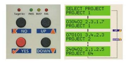
The programmer is capable of performing a multi-project Programming Sequence in Standalone Mode as follows:
