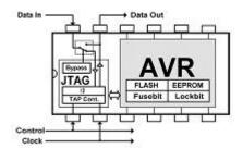
The FS2009USB supports programming of the Atmel ATmega AVR Microcontroller Family using the JTAG algorithm. This chargeable upgrade allows the FS2009 to program the ATmega devices at high speed via the JTAG port of the Target Device.
