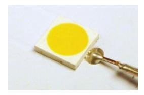
Figure 8. Photo showing representative placement of TC wire secured with thermal conductive epoxy. The thermal epoxy volume should be kept to minimum as shown.
