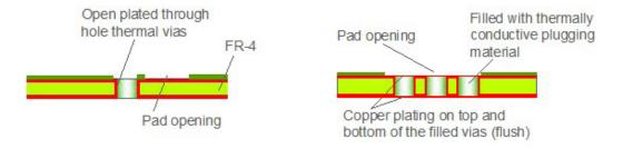
Figure 5. Left picture shows a cross section of an open via with plated through hole design with one pad opening where the LED pad is soldered onto. Right picture shows a cross section of a filled and cap via design with one pad opening. One of the LED pads is then soldered on top of the flush area where the filled and capped vias are underneath it to create direct thermal path connection between LED and bottom of PCB.
