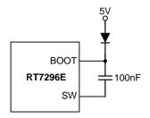
Figure 2. External Bootstrap Diode
