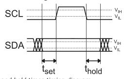
Setup and hold times timing diagram
