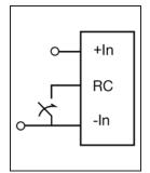
The device should be capable of sinking 0.7 mA. When the RC pin is left open, the voltage generated on the RC pin is max 6 V. The standard product is provided with "negative logic" remote control and will be off until the RC pin is connected to the
