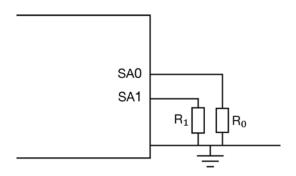
Schematic of connection of address resistors.
