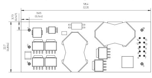
NOTES PIN SPECIFICATIONS Pin 1-5 & 16 Material: Copper alloy Plating: Min Au 0.1 µm over 1-3 µm Ni. Pin 6-15 Material: Brass Plating: Min Au 0.2 µm over 1.3 µm Ni. Pin 6-15 are optional and only used if digital communication is required. Pin position 3 not present due to case to ground pin not available
