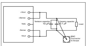
Output ripple and noise test setup
