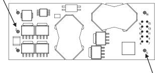
Pin 5 for measurement of minimum pin (solder joint) temperature, T<sub>DIN</sub>
