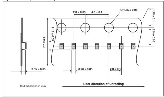
Figure 12. Tape and reel specification
