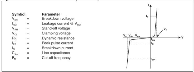
Table 2. Electrical characteristics ( $T_{amb} = 25^{\circ} C$ )
