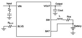
Figure 6. Battery level voltage shift setting circuit
