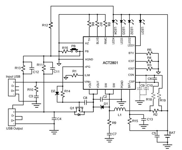
Figure 22. Typical application circuit (Input current limit 2.0A, fast charge current limit 1.5A, boost output constant current limit 1.3A)
