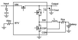
Figure 5. Battery terminal voltage setting circuit
