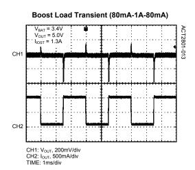
SW and Output Waveforms in Boost Mode
