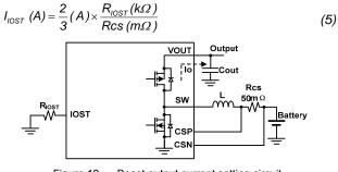
Figure 12. Boost output current setting circuit
