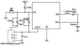
Figure 16. Boost output auto detection circuit
