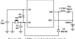
Figure 19. LEDs on in boost mode circuit
