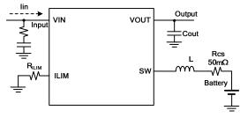
Figure 7. Input current limit setting circuit
