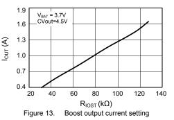
The IOST pin voltage is proportional to output current until output current is limited, as shown in Figure 14.
