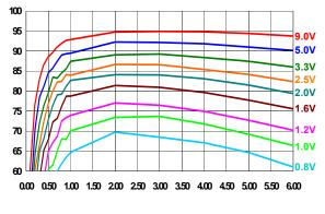
FIGURE 17. ISL6549LOW-EVAL1 MEASURED EFFICIENCY, WITH  $V_{IN1}$  = 12V, @575kHz, AT MULTIPLE OUTPUT VOLTAGES
