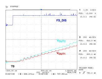
FIGURE 5. ISL6549EVAL1 NORMAL START-UP DETAIL
