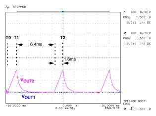
FIGURE 8. ISL6549EVAL1 UNDER-VOLTAGE PROTECTION
