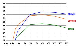
FIGURE 18. ISL6549LOW-EVAL1 MEASURED EFFICIENCY, V<sub>OUT1</sub> = 5V, AT SEVERAL SWITCHING FREQUENCIES
