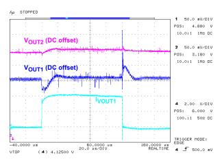
FIGURE 14. ISL6549EVAL1 LOAD TRANSIENT RESPONSE
