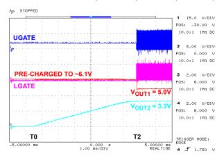
FIGURE 7. ISL6549EVAL1 START-UP INTO AN OVER-CHARGED OUTPUT
