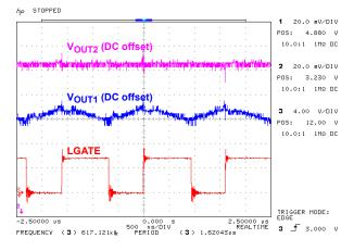
FIGURE 13. ISL6549LOW-EVAL1 OUTPUT SWITCHING RIPPLE VOLTAGE
