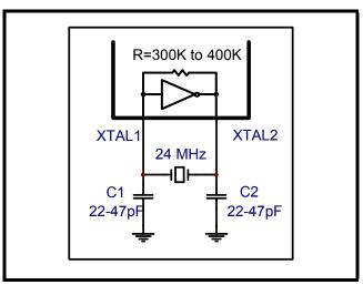
FIGURE 3. TYPICAL OSCILLATOR CONNECTIONS
