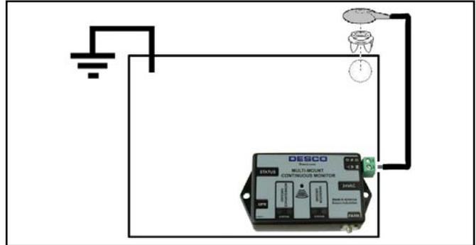
Figure 4. Installation method #2 of the Multi-Mount Continuous Monitor
