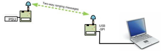
Using one of the EVBs as a portable device enables you to more easily evaluate performance on range, accuracy, LOS & NLOS situations, immunities etc...
