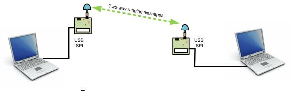
The PC DecaRanging application allows you to run a two-way ranging demo on two PCs/Laptops simply by using the USB-SPI connectivity provided on the EVB1000.
