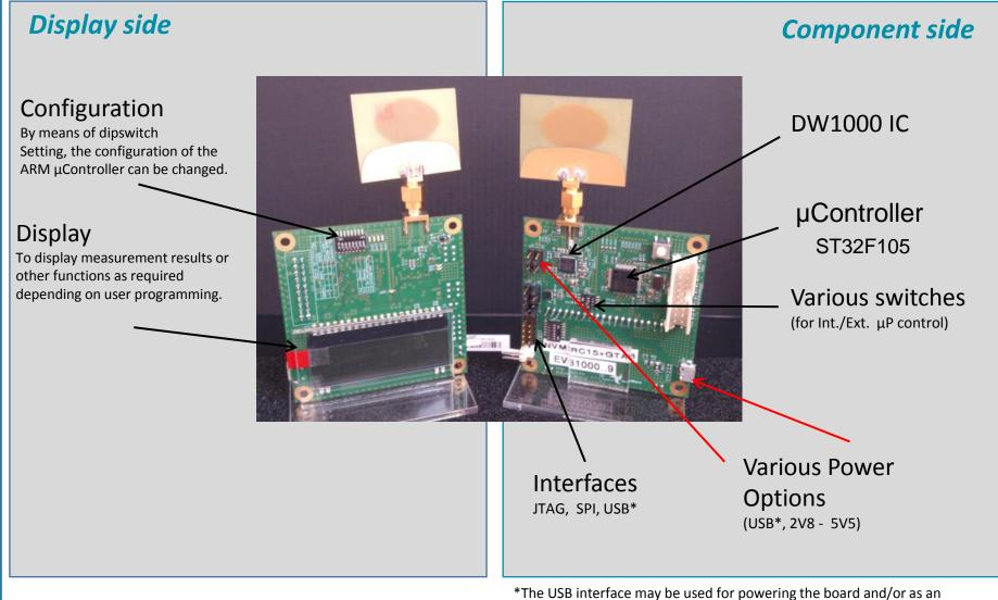
\*The USB interface may be used for powering the board and/or as an optional means to drive the DW1000 IC from an external PC (instead of using SPI Interface)
