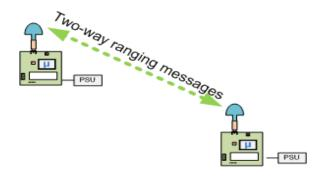
The EVK1000 provides all HW and SW elements to perform a Two-Way Ranging evaluation, including: Range accuracy, Range precision, Range sensitivity, Multipath immunity, Blocking immunity and much more.
