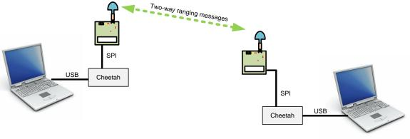
Similar to the above configuration but using Cheetah's to connect to the SPI port on the DW1000
