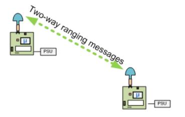
Once communication is established between the two nodes and ranging commences, the display on each node shows last measured range and an average of the last 8 measurements
