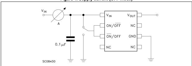
Note: The switch emulates two possibilities to set the regulator in OFF mode.
