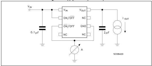
Figure 4. Supply current (OFF mode)
