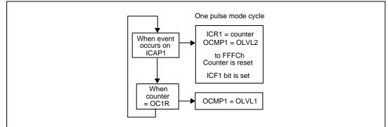
When a valid event occurs on the ICAP1 pin, the counter value is loaded in the ICR1 register. The counter is then initialized to FFFCh, the OLVL2 bit is output on the CCiviP1 pin and the ICF1 bit is set.
