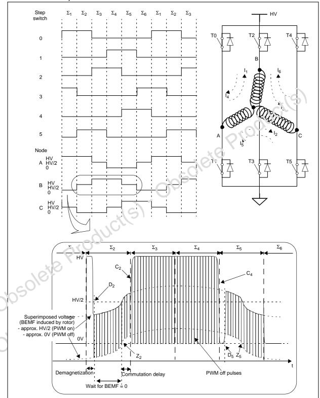
Figure 75. Example of command sequence for 6-step mode (typical 3-phase PM BLDC motor control)
