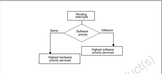
When an interrupt request is not serviced immediately, it is latched and then processed when its software priority combined with the hardware priority becomes the highest one.
