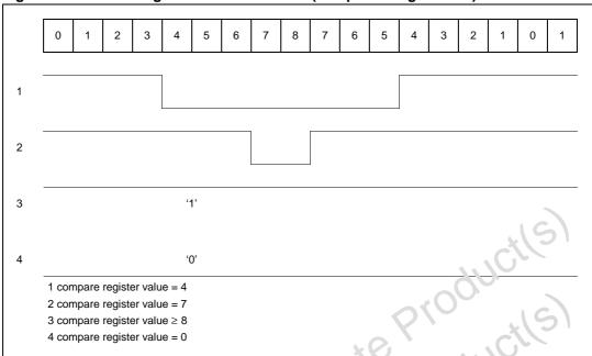
Figure 120. Center-aligned PWM waveforms (compare 0 register = 8)
