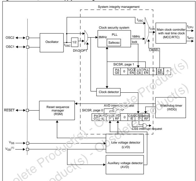
Figure 9. Clock, reset and supply block diagram
