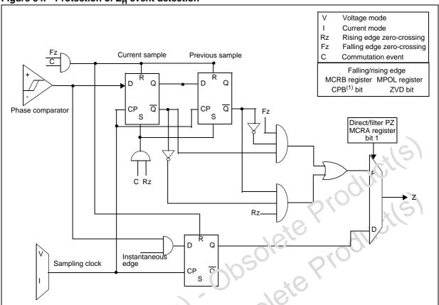
Figure 84. Protection of Z<sub>H</sub> event detection
