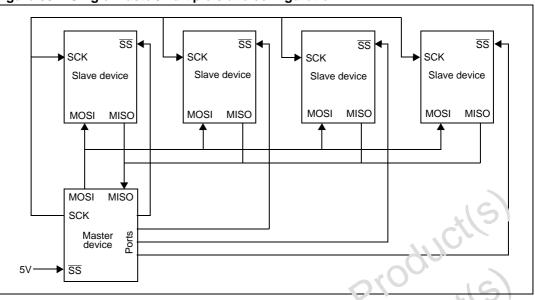
Figure 60. Single master/multiple slave configuration
