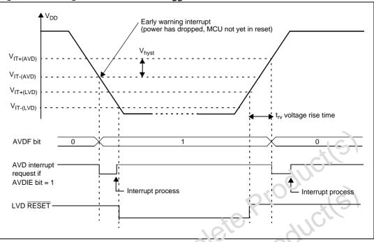
Figure 14. Using the AVD to monitor V<sub>DD</sub>
