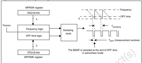
Figure 108. Sampling clock generation block<sup>(1)</sup>
