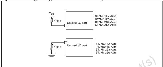
Figure 139. Two typical applications with unused I/O pin
