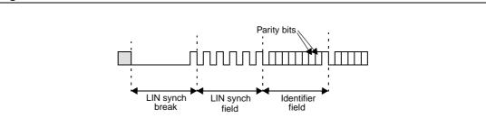
The bits involved are the two MSB positions (7th and 8th bits if M = 0; 8th and 9th bits if M = 0) of the identifier character. The check is performed as specified in *Figure* 67 by the LIN specification.
