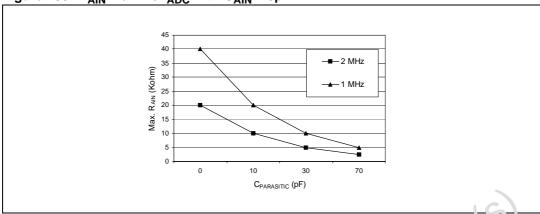
$C_{\mathsf{PARASITIC}}$  represents the capacitance of the PCB (dependent on soldering and PCB layout quality) plus the pad capacitance (3pF). A high  $C_{\mathsf{PARASITIC}}$  value downgrades conversion accuracy. To remark this,  $f_{\mathsf{ADC}}$  should be reduced. 1.
