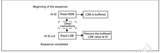
The user must read the MSB first, then the LSB value is buffered automatica";
