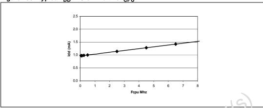
Figure 135. Typical I<sub>DD</sub> in Slow Wait vs f<sub>CPU</sub>
