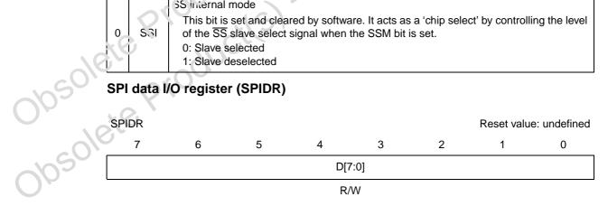
The SPIDR register is used to transmit and receive data on the serial bus. In a master device, a write to this register initiates the transmission/reception of another byte.
