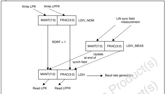
Figure 71. LDIV read/write operations when LDUM = 1
