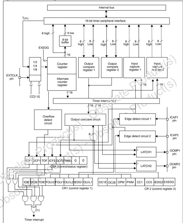
Figure 40. Timer block diagram
