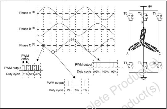
Figure 77. Typical command signals of a three-phase induction motor
