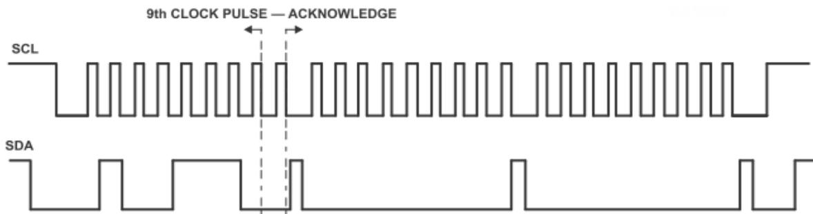
Figure 12: Bus A (0.6V to 5.5V Bus) Waveform
