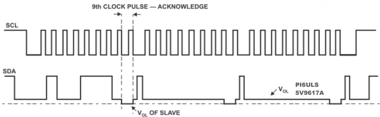
Figure 13: Bus B (2.2V to 5.5V Bus) Waveform
