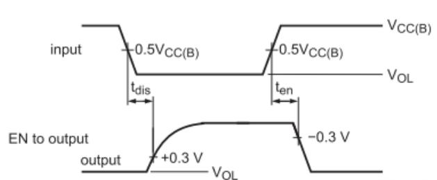
Figure 7: Propagation Delay and Enable and disable time
